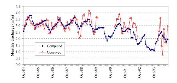
Figure 12: Computed and observed discharge series at Melas springs.
