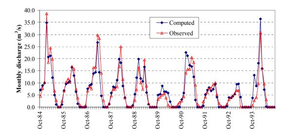
Figure 7: Computed and observed discharge series at the basin outlet.
