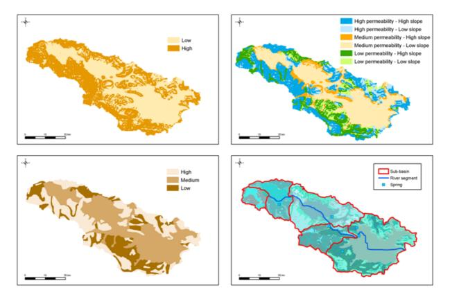
Figure 4: Characteristic layers of geographical data for the schematisation of the surface system: (a) top left, terrain slope; (b) bottom left, permeability; (c) top right HRUs, derived as the product of slope and permeability; (d) bottom right, product of HRUs and sub-basins.
