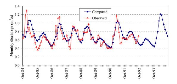
Figure 11: Computed and observed discharge series at Herkyna springs.
