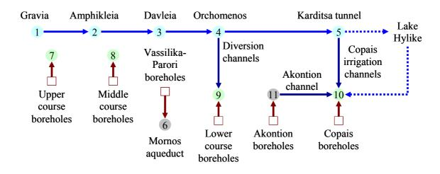
Figure 6: Simplified sketch of the water management network, representing abstractions from the surface and groundwater resources. Nodes 1-5 are river points, whereas nodes 7-10 denote agricultural areas across the basin.
