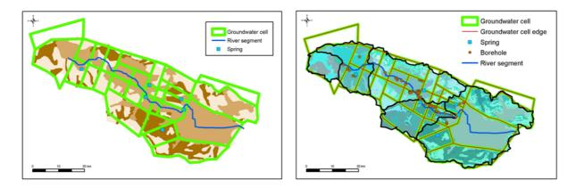
Figure 5: Characteristic layers of geographical data for the schematisation of the groundwater system: (a) left, formulation of cells, based on permeability; (b) right, product of cells, sub-basins, HRUs, springs and boreholes.
