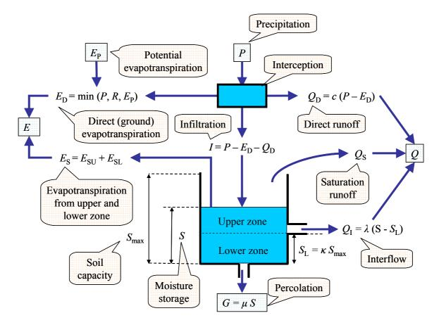
Figure 1: Schematic layout of the surface water balance model.
