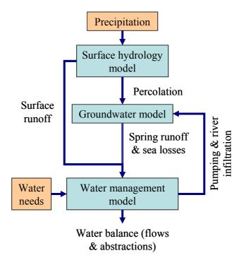
Figure 2: Simulation flowchart, explaining the co-operation of the three models.
