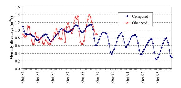
Figure 13: Computed and observed discharge series at Polygyra springs.
