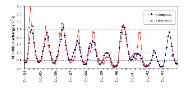
Figure 8: Computed and observed discharge series at Lilaia-Kefalovrysso springs.
